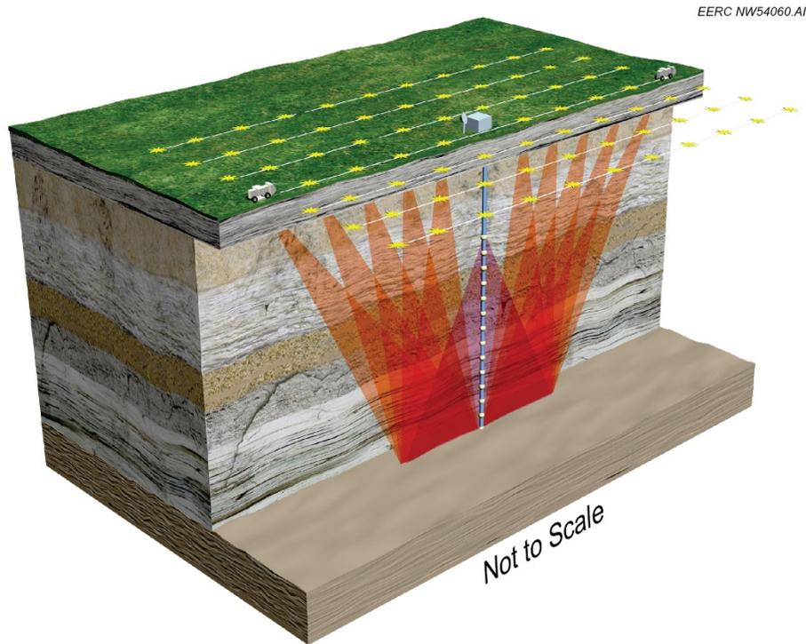
Figure 10. Schematic of VSP survey (Hamling and others, 2011).
