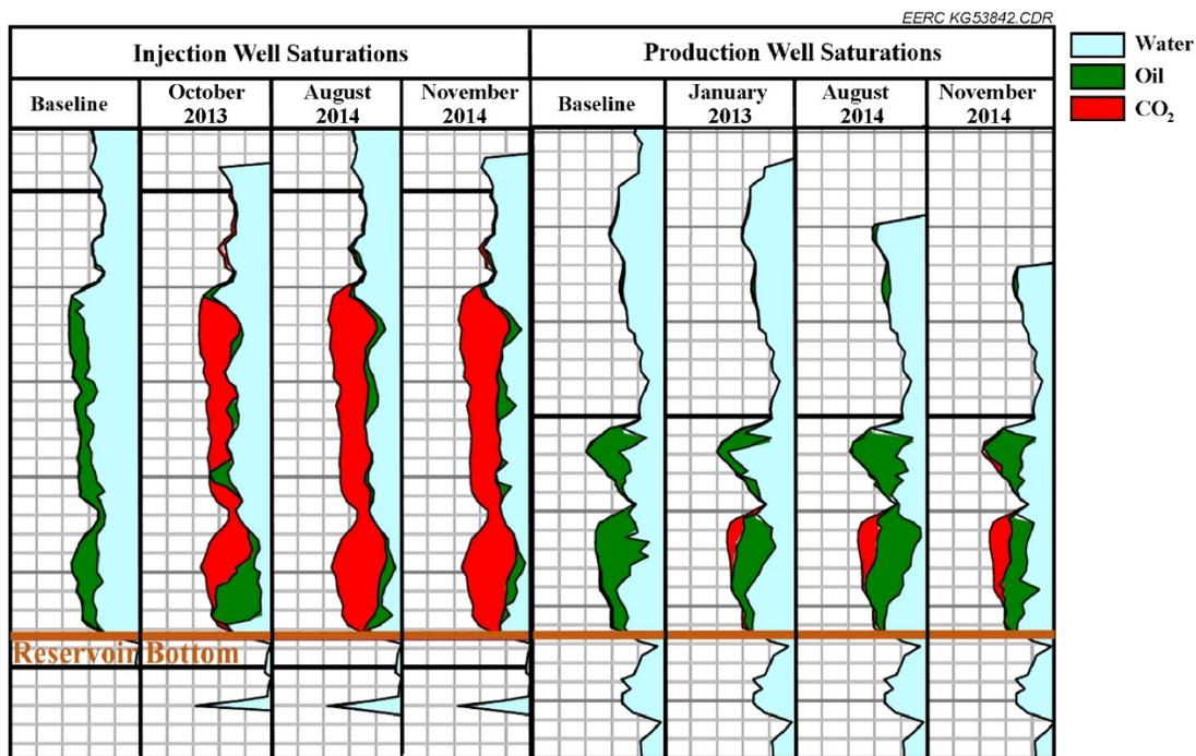
Figure 5. Time series of PNLs showing changes in fluid saturations in the reservoir interval between baseline and repeat campaigns for three injection wells and one production well.
